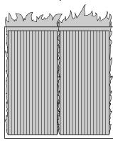
Figure 21 - Incorrect Burner Flame Pattern (Model VN10 Shown)
